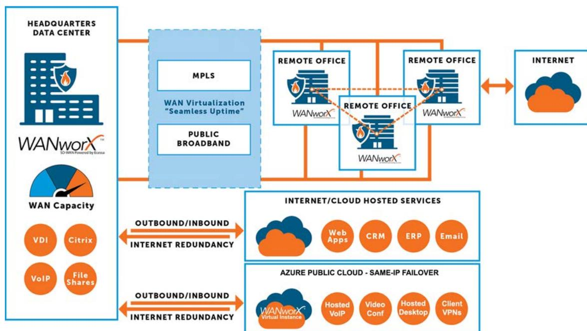
*This solution uses a local Ecessa WANworX® appliance and a virtual instance of Ecessa software running on a virtual machine (VM) in the Azure Public Cloud.*
