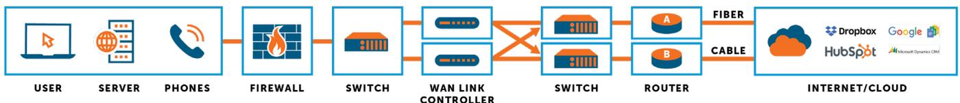
When hardware is configured as a High Availability (HA) pair, the failover mechanisms run in the background, so the transfer takes place automatically. There is no need to drive to the office in the middle of the night to manually connect and configure replacement hardware. The data on both systems is continuously and automatically synchronized. To the user, failover resembles a very fast automatic service reboot.
