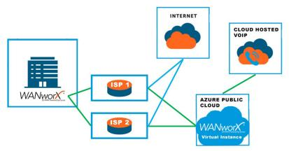
As you can see, the solution requires a local Ecessa WANworX appliance and a virtual instance of Ecessa software running on a VM in the Azure Public Cloud. While the Ecessa WANworX appliance is a fixed cost, the virtual instance pricing can vary, based on the resources allocated to the VM and the bandwidth used.
