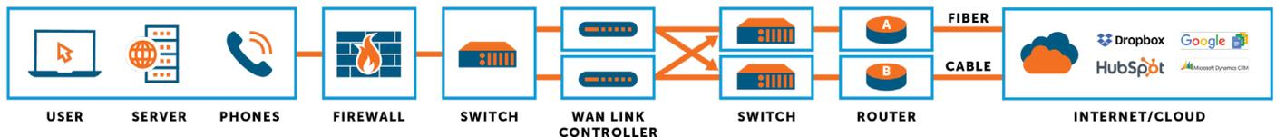
The capability to switch automatically to a redundant or standby system or network upon failure happens without human intervention (see Failover Hierarchy for other types of failover). Automated failover is essential in servers, systems or networks requiring continuous availability and a high degree of reliability — those responsible for mission-critical processes and data.
