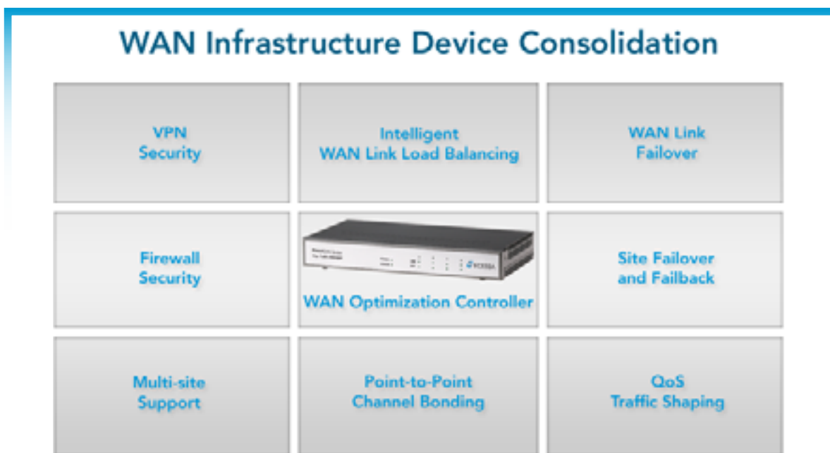
This diagram shows some of the technology consolidation that WAN link controllers are providing
